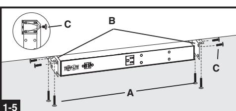
**1-4 Wall Installation.** After repeating Part 1 above, attach the PDU to a stable mounting surface by inserting two or more user-supplied screws (A) through the PDU mounting brackets (B) and into secure mounting points on the mounting surface.
