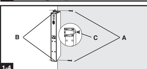
**1-3 0U Rack Installation.** Part 1: Remove the screws (C) attaching the mounting brackets to the PDU, change the orientation of the brackets as shown and reattach the brackets. Use only the screws supplied by the manufacturer or their exact equivalent (#6-32, 1/4" flat head). Part 2: Attach the PDU vertically by inserting two or more user-supplied screws (A) through the PDU mounting brackets (B) and into mounting points in the rack or rack enclosure.
