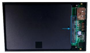
Using the included Philips head screw driver, attach your 2.5" SATA HDD/SSD to the
