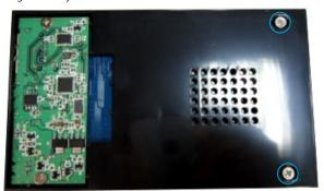
4. Slide the hard drive tray back inside the enclosure.
