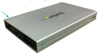
Complete installation by connecting your hard drive enclosure to your computer using eSATA/eSATAp or USB 3.0.
