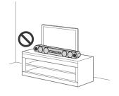
Place the subwoofer at least 10 cm from the wall to avoid damaging the protruding AC power cord (mains lead).
