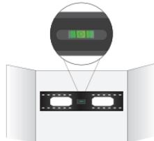
4 .- Place the backplate on the wall, insert the screws (M) and washers (K) in the anchors tighten firmly.
