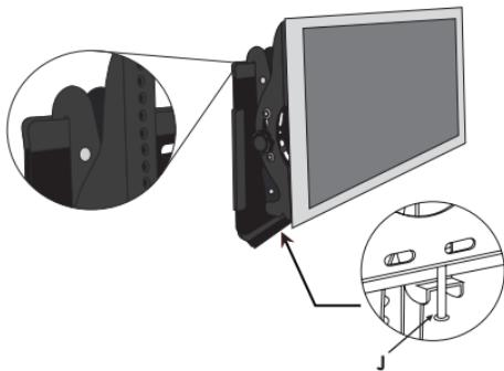
6.- Place the screw (J) which allows horizontal movement and tighten until firm.
