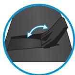
3. The keyboard's inclination angle may be adjusted by pulling out the two tabs located at the bottom.
