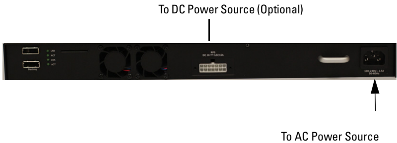
Figure 1-11. AC and DC Power Connection to an N2048 Switch
