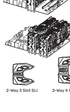
Install your first GeForce® graphics card into the Primary PCIe x16 slot (the Primary slot is the one closest to the CPU).
