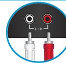
2. Connect an RCA cable from the converter's audio output to the input of your audio player.
