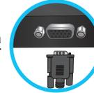
3. Connect the VGA cable to the converter output and to the monitor or display.
