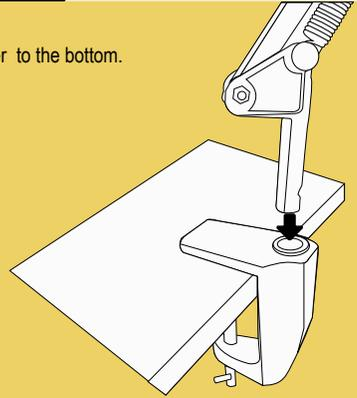
3. Adjust the lamp at the points indicated, until you reach the desired position. Squeeze the nuts to secure the position.
