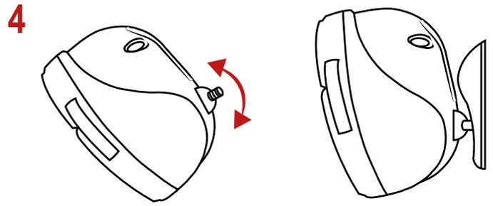
Adjust the position of the speaker and tighten the screws when the angle is right.
