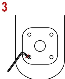
Loose the screws with an allen wrench
