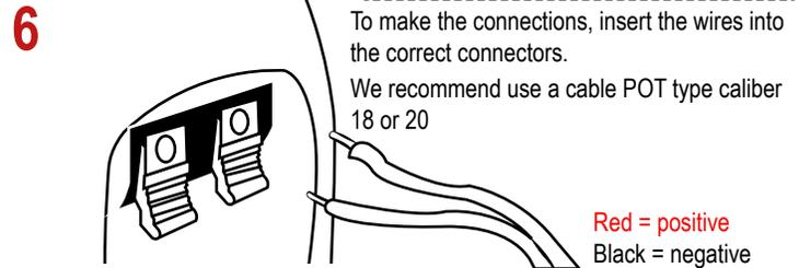
To make the connections, insert the wires into the correct connectors. We recommend use a cable POT type caliber 18 or 20
