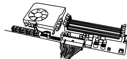
Insert the **SATA** connector into te drivers or optical drivers.
