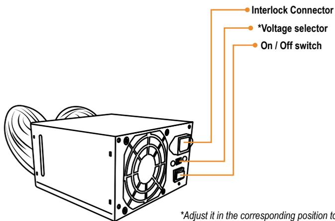
*\*Adjust it in the corresponding position to the AC voltage (230V - 115V) in which the power supply will work.*
