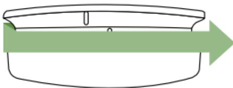
Pull up the battery's compartment cover and insert a 9V battery.
