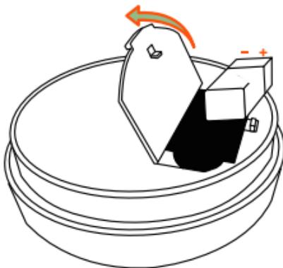
Ensure that the polarity is correct.
