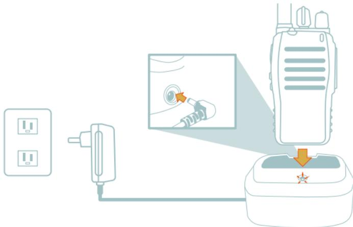
*During the charge process the indicator LED will remains turn on in red color; will change to green when the battery will charge fully.*
