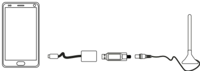
Connect the tuner into the micro USB port of the OTG cable and the micro USB connector in your smartphone. *If you want enter to the app automatically each time that you connect your Smart Tuner ; press **OK**.*
