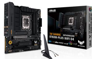
LGA 1700, Intel B760 Chipset, 4 x DDR4-SDRAM up to 128GB, LAN, WLAN, 1 x RJ-45, 4 x SATA III, 2 x M.2(M), UEFI AMI, Micro ATX
