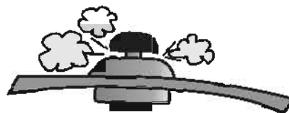
Figure 6. Overpressure Valve Releasing Steam
