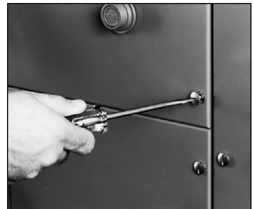
Figure 50: Loosening Captive Quarter-turn Fasteners
