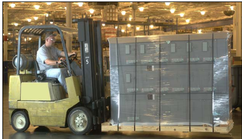
Figure 2: Moving the MCC with a Fork Truck
