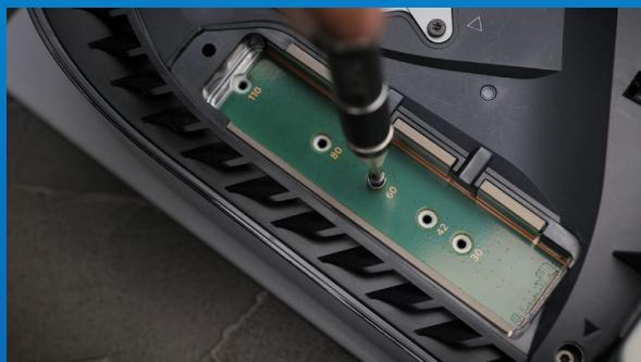
**REMOVE THE SINGLE SCREW AND THE WASHER-LIKE STANDOFF UNDERNEATH.**
