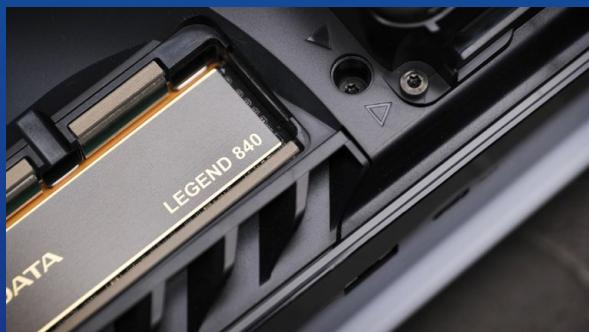
**CLICK THE GOLD CONNECTOR OF THE SSD INTO THE MATCHING INPUT NOTCH.**
