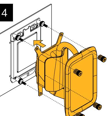
Hold waterblock in place and attach mounting nuts (E)
