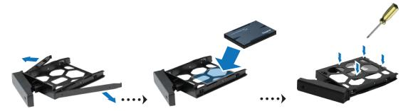
**4** Insert the loaded hard drive tray into the empty hard drive bay and push it into position by the upper half of the handle.
