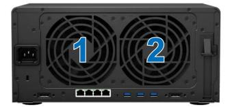
3 Remove the four screws that secure the fan panel.
